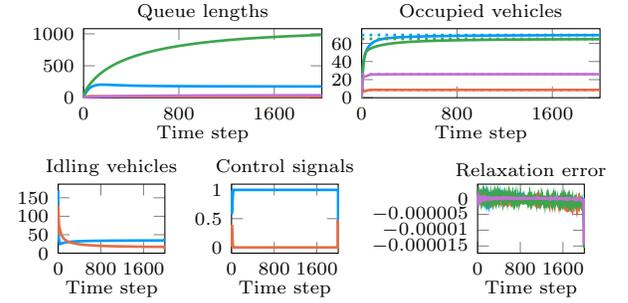
Fig. 3. The trajectories with the MPC for the high demand scenario. For the occupied vehicles, the dotted lines represent the equilibrium. For legend description, see Fig. 2.
